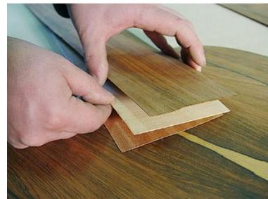
The main purpose of the sides of a classical guitar body are to provide strength and rigidity to the instrument and laminates are ideal for this. Three-ply laminates have the grain of at least one layer running in across the grain of the other layers, and this gives the construction great strength and rigidity. A guitar made with laminated sides will be hardy and not at all likely to crack, at least not on its side panels.
